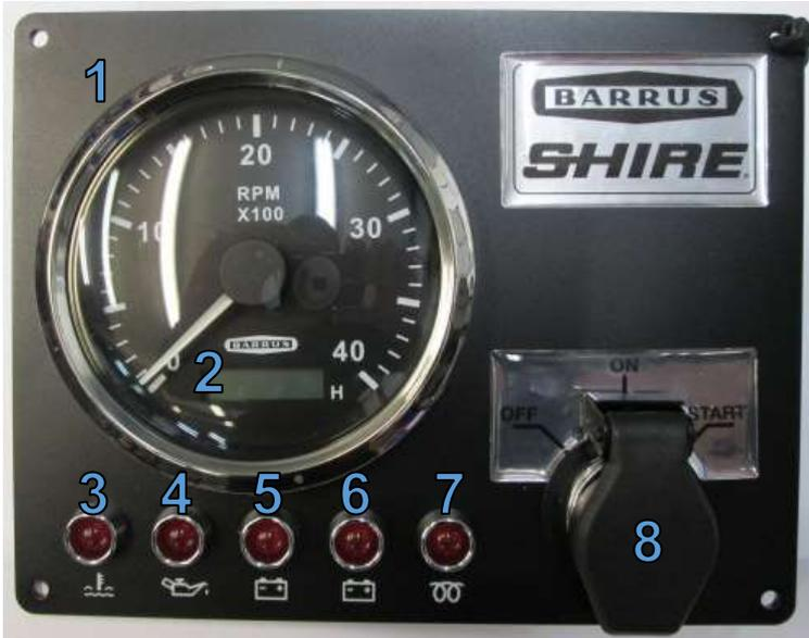
Figure 12: Standard Control Panel
