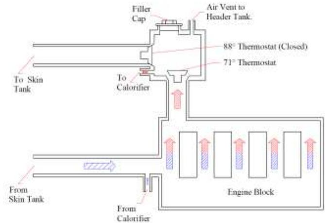
If the load on the engine reduces and the demand for domestic hot water increases then the system will automatically compensate and re-direct water to ensure that a plentiful supply of hot water is always available.
