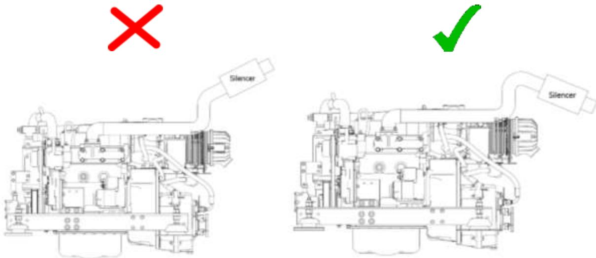
Figure 23: Correct Exhaust Installation
