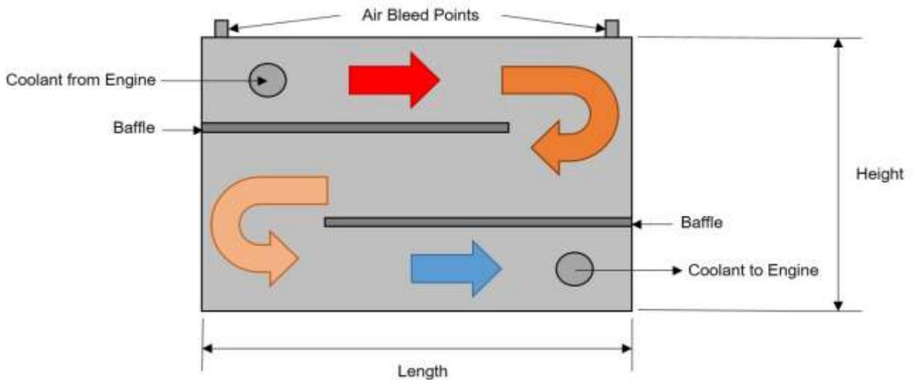
Figure 16: Skin Tank Flow Diagram
