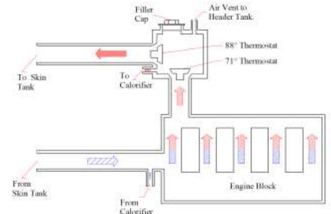
**Figure 24: Twin Thermostat Operation**
