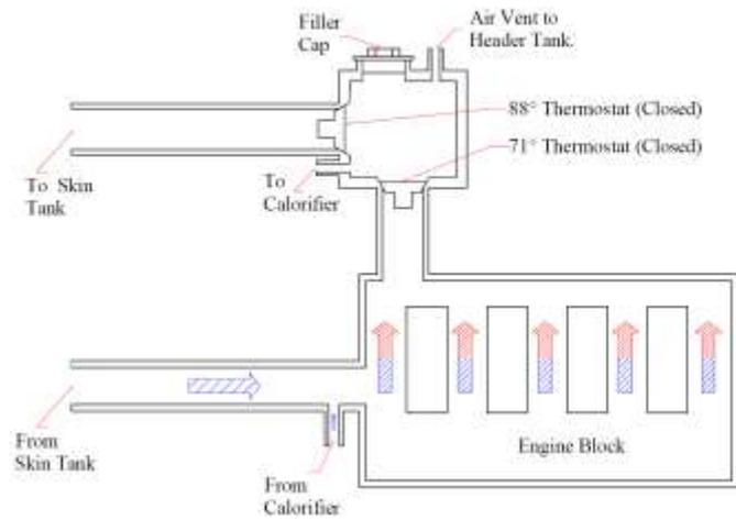
When the water stored in the hot water tank has reached full temperature, the second 88° thermostat opens and water can then flow to the skin tank and correctly control engine cooling. The exhaust manifold that earlier helped to heat engine water is now cooled to ensure safe operation and reduce engine compartment temperatures.
