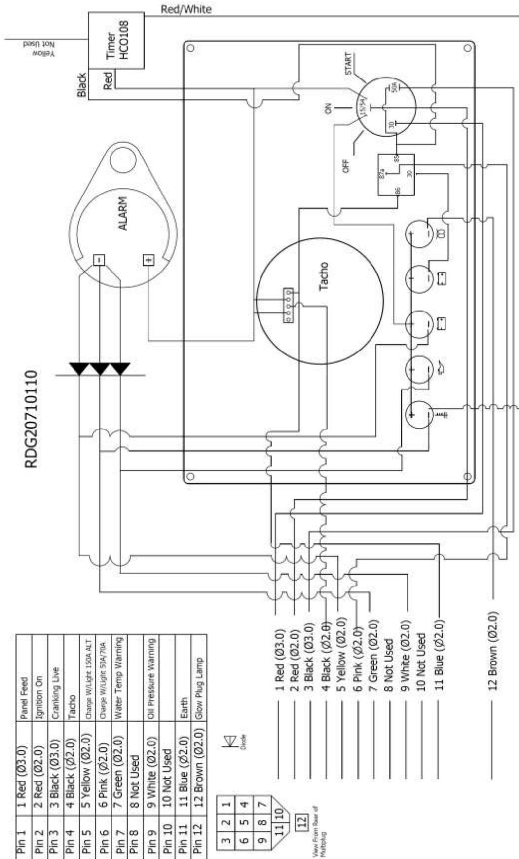
Figure 28: Standard Control Panel Wiring Diagram
