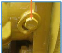
• Loosen the three nuts securing the fuel injection pump to the engine. Make sure the fuel injection pump is in the middle of its adjustment on the slots. When the fuel injection pump is in the middle of the slots retighten the nuts.
