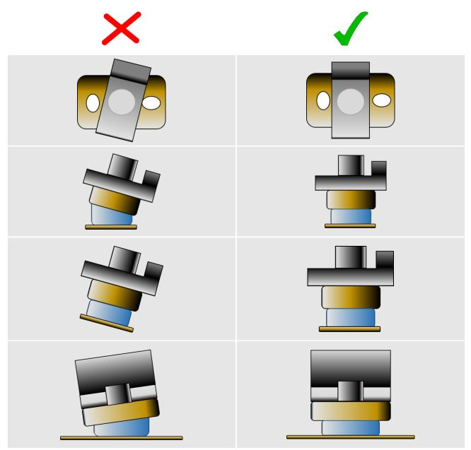
Figure 17: Correct Anti-Vibration Mount Installation
