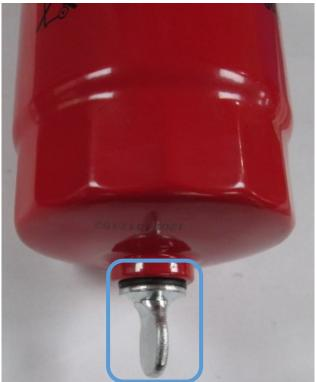
Figure 23: Primary Fuel Filter Drain Screw
