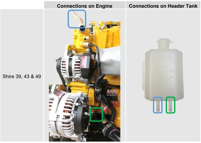
Figure 15: Header Tank Connections
