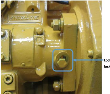
Lock pin in the locked position
