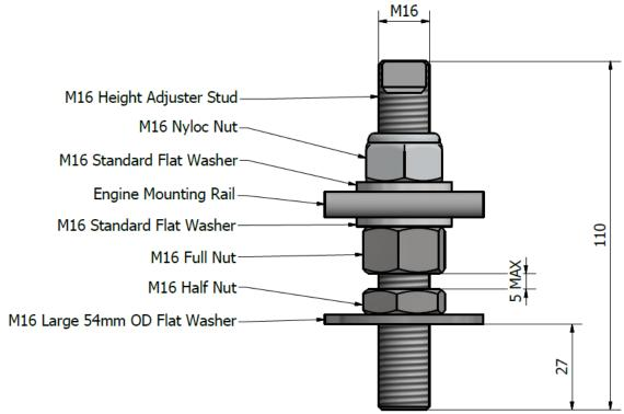
Figure 18: Correct Anti-Vibration Mount Installation
