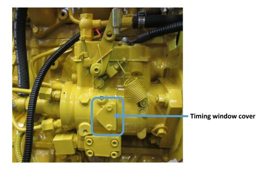
• Make sure the line on the shaft and the line on the pump body line up.
