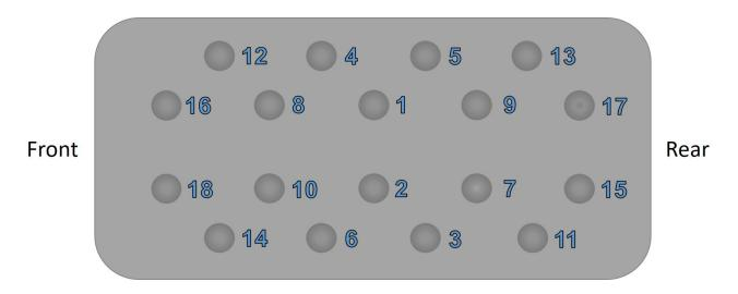
Figure 31: Cylinder Head Tightening Sequence
