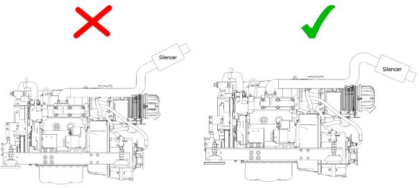
Figure 21: Correct Exhaust Installation
