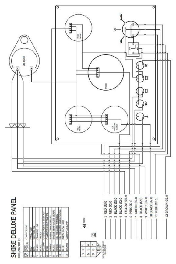
Figure 29: Deluxe Control Panel Wiring Diagram
