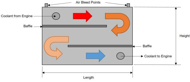
Figure 14: Skin Tank Flow Diagram
