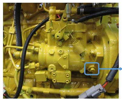
Lock pin in the unlocked position
