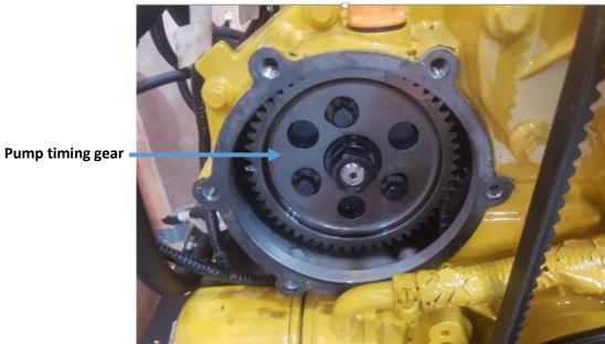
Put the timing lock pin on the fuel injection pump back into the unlocked position. •
