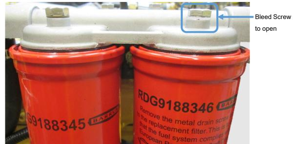
Figure 24: Fuel Filter Bleed Screw
