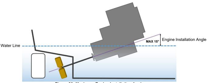
Figure 20: Maximum Engine Installation Angle
