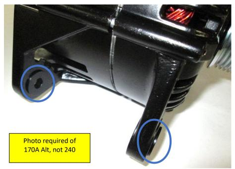
• Fit the 170A Alternator assembly to the Alternator Bracket securing with M10 Nyloc Nuts (RDG2106 x 2), M10 Flat Washers (RDG628 x 4), M10 x 50 Hex Head Bolt (RDG3940 x 1) and M10 x 55 Hex Head Bolt (RDG5373 x 1). The spare washers can be used to space out the alternator if required. NOTE: Don't tighten the screws at this stage.
